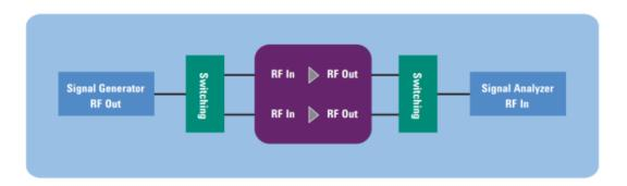
The combination of the RF cables and the switching network can add several dB of loss between the output of the M9381A PXIe VSG and the input of the DUT, which requires higher output levels from the M9381A PXIe VSG. Since the tests are performed with a modulated signal, the M9381A PXIe VSG must also have adequate modulation performance at the higher power levels.
