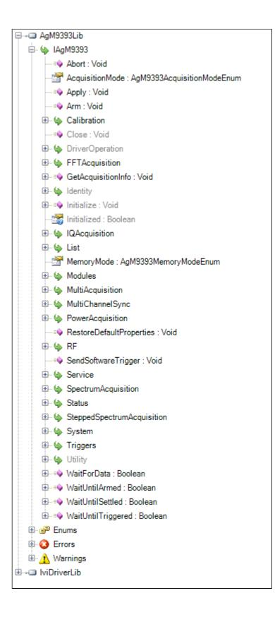
The following table lists the instrument-specific hierarchy interfaces for M9393A PXIe VSA:
